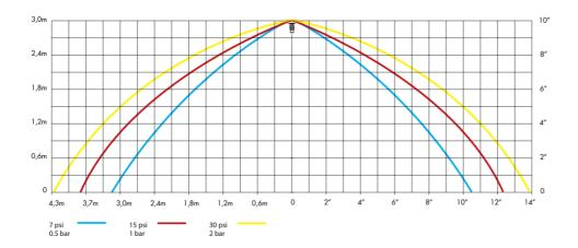
**SIDEWALL K 5.6 SPRINKLER** DY-3329/ DY-3339 / DY-3429 / DY-3439
